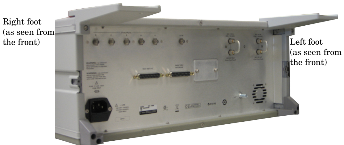
Figure 9 Install Locking Feet on N5261/62A
